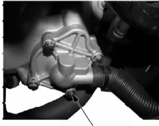
Bolts of draining + sealing shim
