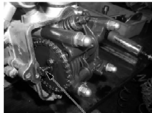
oil channel joint and spring
