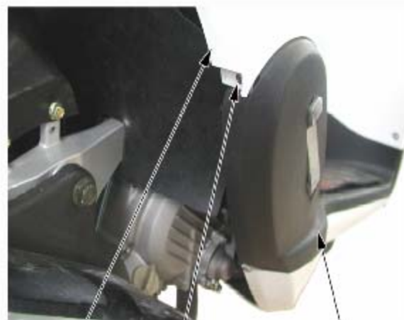
self tapping screw 3 right guard board right heel of foot board
