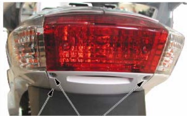
rear connecting board self tapping screw 1
