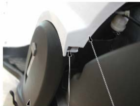
self tapping screw 2 left heel of foot board left guard board
