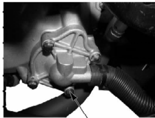
Bolts of draining + sealing shim
