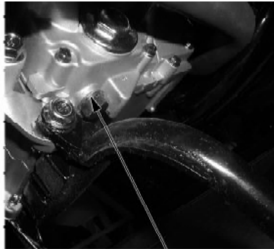
drain bolt sealing gasket
