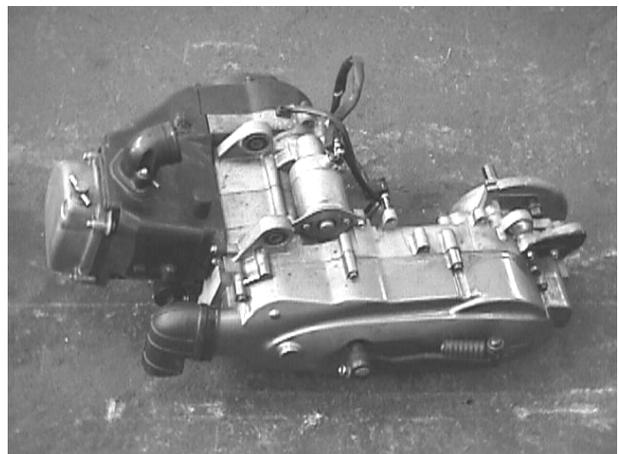
**(1) Drive pulley, starter clutch. driven pulley**
