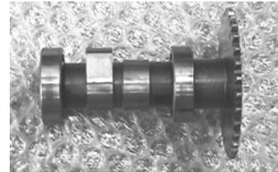
Check camshaft. If the bearing is loosen or worn out, change the whole set if necessary.
