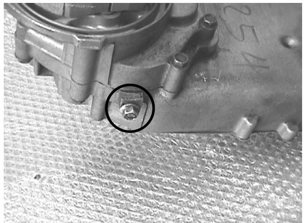
3. Remove the bolt in the gear box cover.
