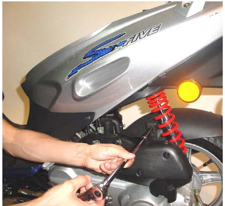
**Before removing make sure to disconnect the rubber hose that is connected to the air box.
