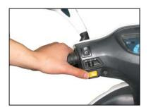
• When key is on, pressing button will sound horn.
