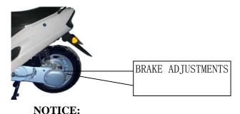
• After brake adjustment match the concavity of the adjusting nut with the axle pin to prevent the change of free play during riding.
