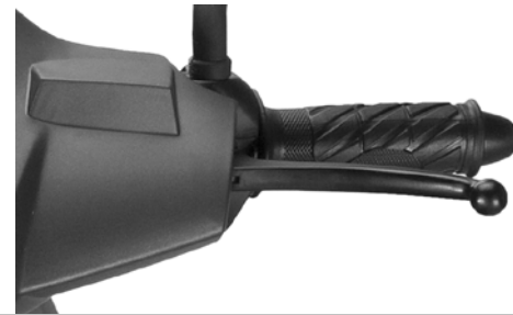
Rear brake handle: When applied, the rear brake will engage and slow the vehicle.
