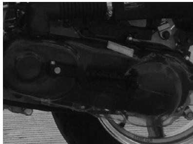
Automatic clutch: The belt driven CVT transmission allows for constant acceleration with no need for gear changes. Simply turning the throttle will engage the transmission.
