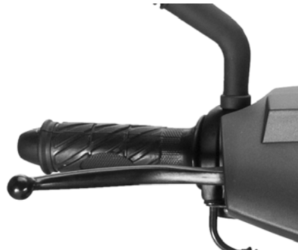
Front brake handle: When applied, the front brake will engage and slow the vehicle.
