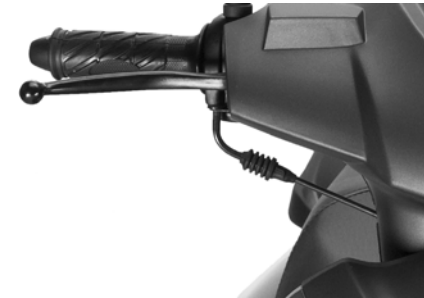
Adjust the free travel of the front braking handgrip between 1/4 and 1/2 inch
