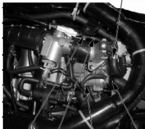
locknut gun guy cable water-recycled pipe and hoop water outlet pipe and hoop
